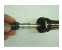
The fork cartridges will now be filled with oil and bled of any air.
