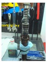
On some cartridges and models, the compression valve may seem to only go in half way until it feels like it hydraulically stops, this is normal.
